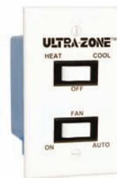
Remote selector switch for use with ST series ULTRA-ZONE Control panels. This switch replaces the zone 1 thermostat subbase if separate remote system control is desired. 4 wires required.
