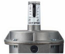
The EBD style by-pass are self-contained units that give you the static control mounted to the damper. It is an “all-in-one” design that makes the installation process much easier than most electronic by-pass dampers. The static pressure can be adjusted in the field between 0.1" to 4" of pressure. This is done by the turn of a set-screw. Requires 24VAC to operate. Tubing and pitot tube are included.
