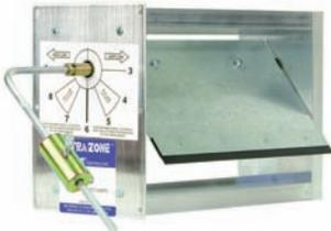
Model PRD pressure regulating damper is a single blade, steel, barometric damper with a counter balanced weighted arm. The PRD provides an economical solution for bypassing excess air when zone dampers close.
