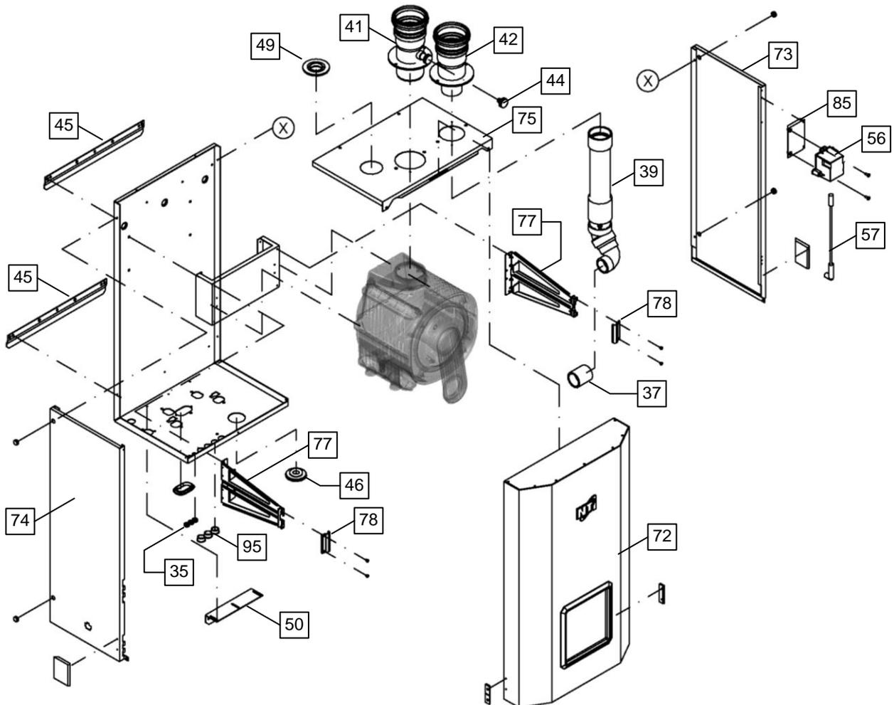
Figure 19-1(d) Tx Controls, Electrical Panel and Display Module
