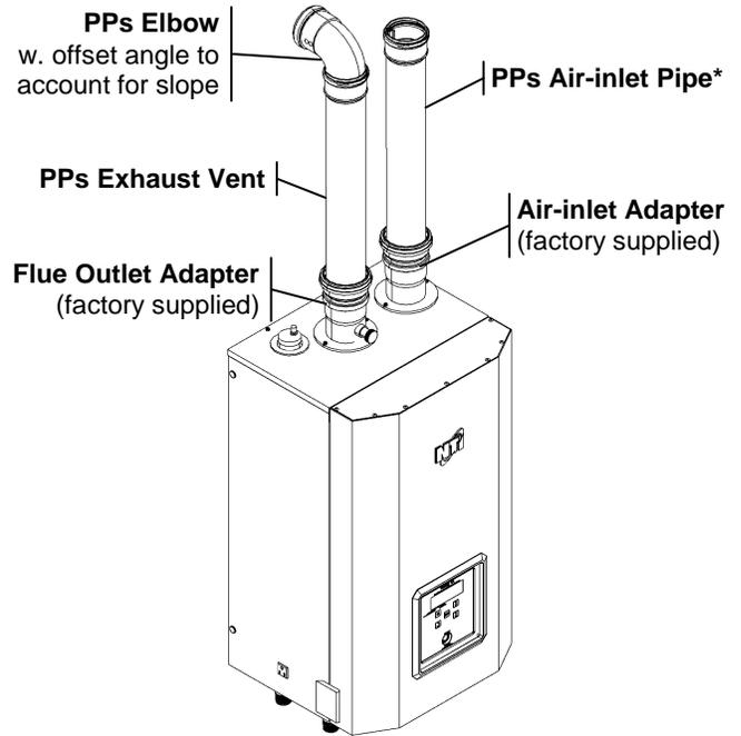
\* Air-inlet - check with applicable local codes for acceptable pipe material.
