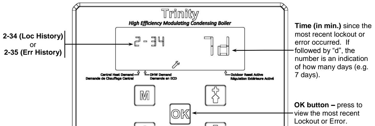
**Figure 17-5b Lockout and Error History Navigation (Submenu)**
