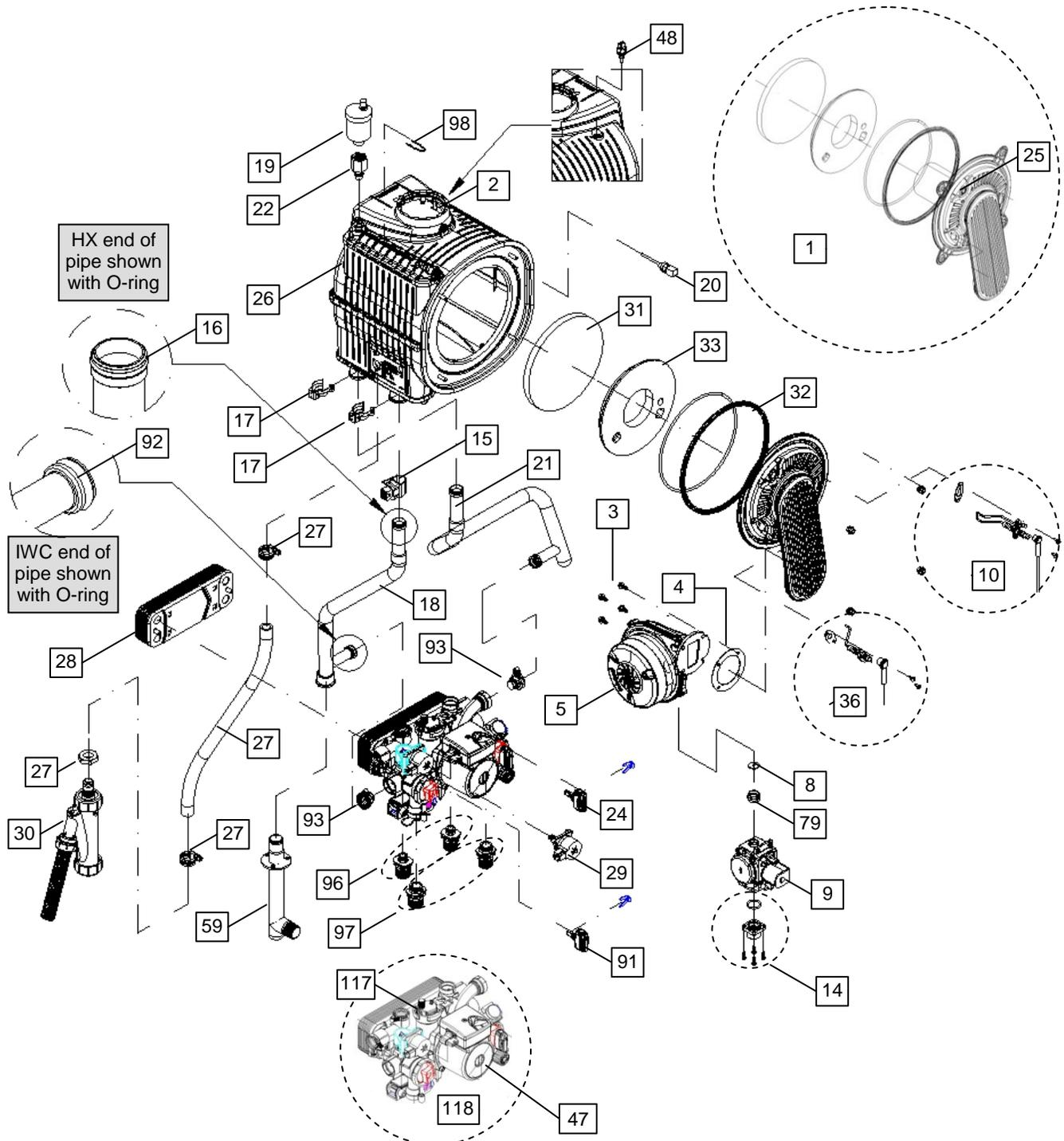
Figure 19-1(b) Tx200 Gas Valve & Blower Assembly
