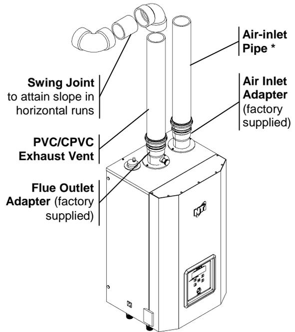
Figure 4-2(b) Near Boiler Vent Connections (PPs – Polypropylene)
