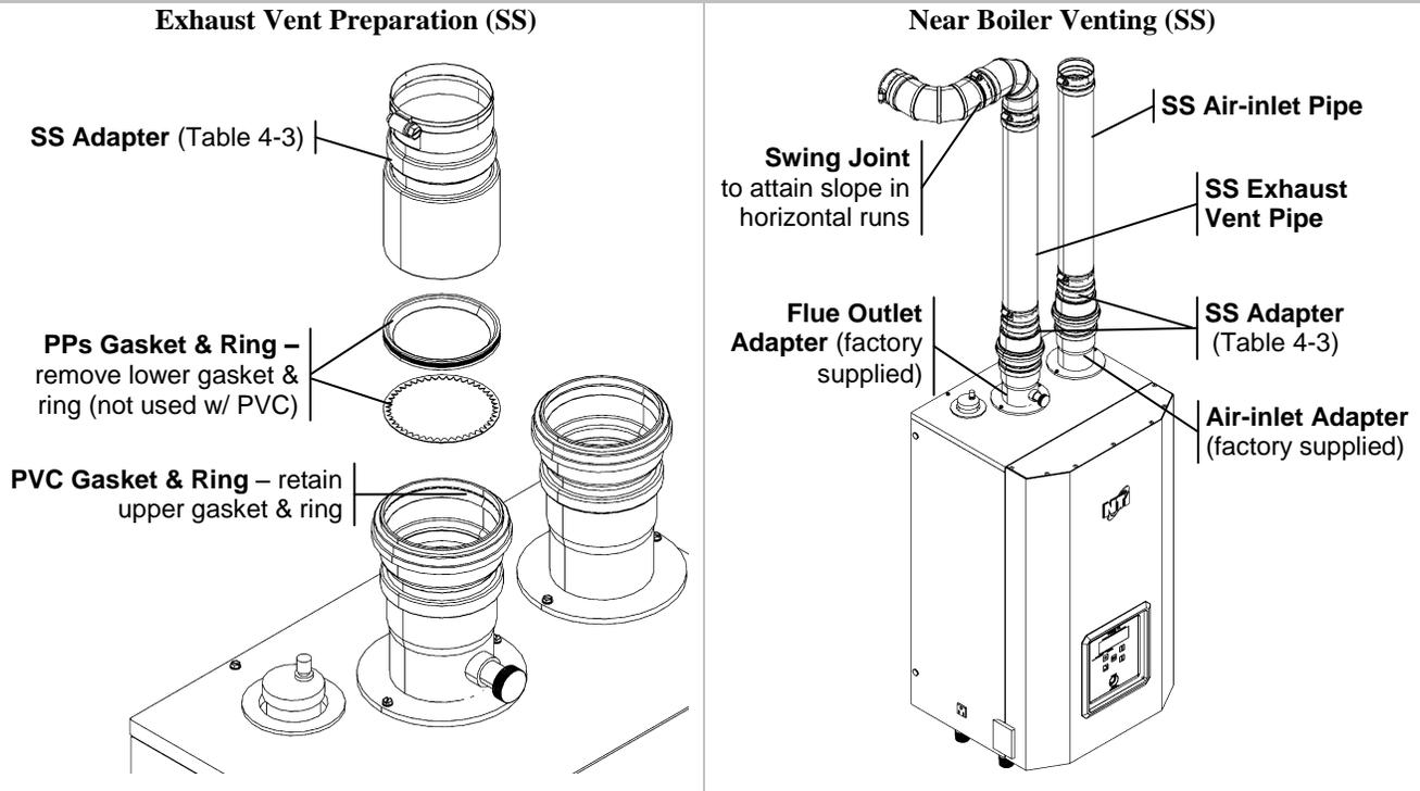
Vent/Air-inlet Pipe Material
