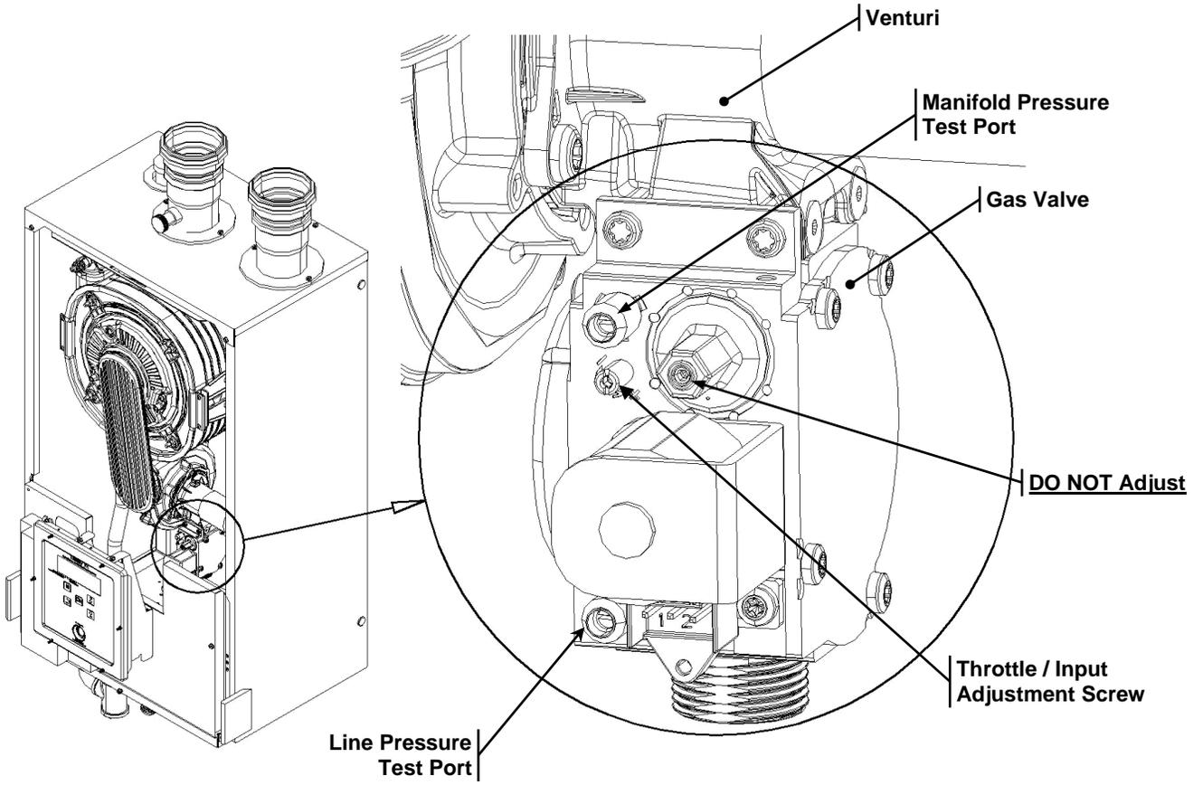
Figure 9-2 Gas Valve and Venturi Assembly (Tx200)
