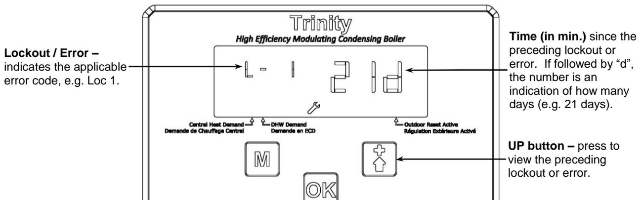
Figure 17-5c Lockout and Error History Navigation (End)
