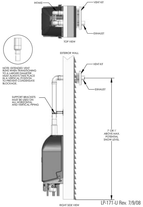
**Fig. 7-10 2" sidewall vent with V500 kit**
