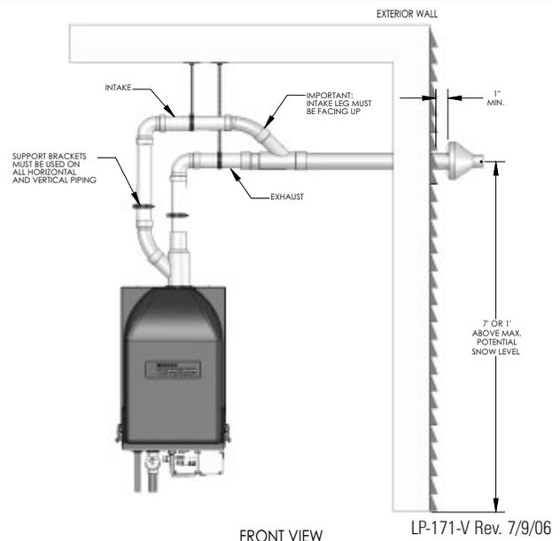
**Fig. 7-11 2" sidewall vent with 2" concentric vent kit (KGAVT0501CVT)**
