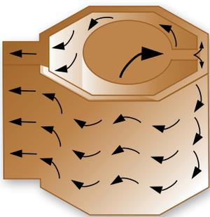
The octatherm heat exchanger’s unique eight sided design provides more efficient use of the heat transfer area. This design puts less stress on the steel and thus provides a longer life. As a result, the octatherm design generates increased dependability and a lifetime of comfort for your home.
